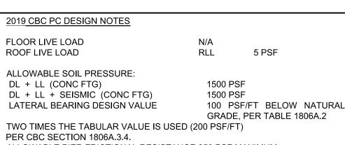
ALLOWABLE PIER FRICTIONAL RESISTANCE 250 PSF MAXIMUM BASED ON SECTION 1810A.3.3.1.4 (ONE-SIXTH OF THE BEARING VALUE). UPLIFT FRICTIONAL RESISTANCE HAVE A SAFETY FACTOR OF 3.
