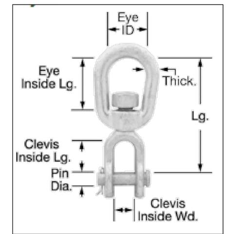
EYE-TO-CLEVIS SWIVEL MATERIAL: GALVANIZED STEEL LENGTH: 5 7/8" EYE:
